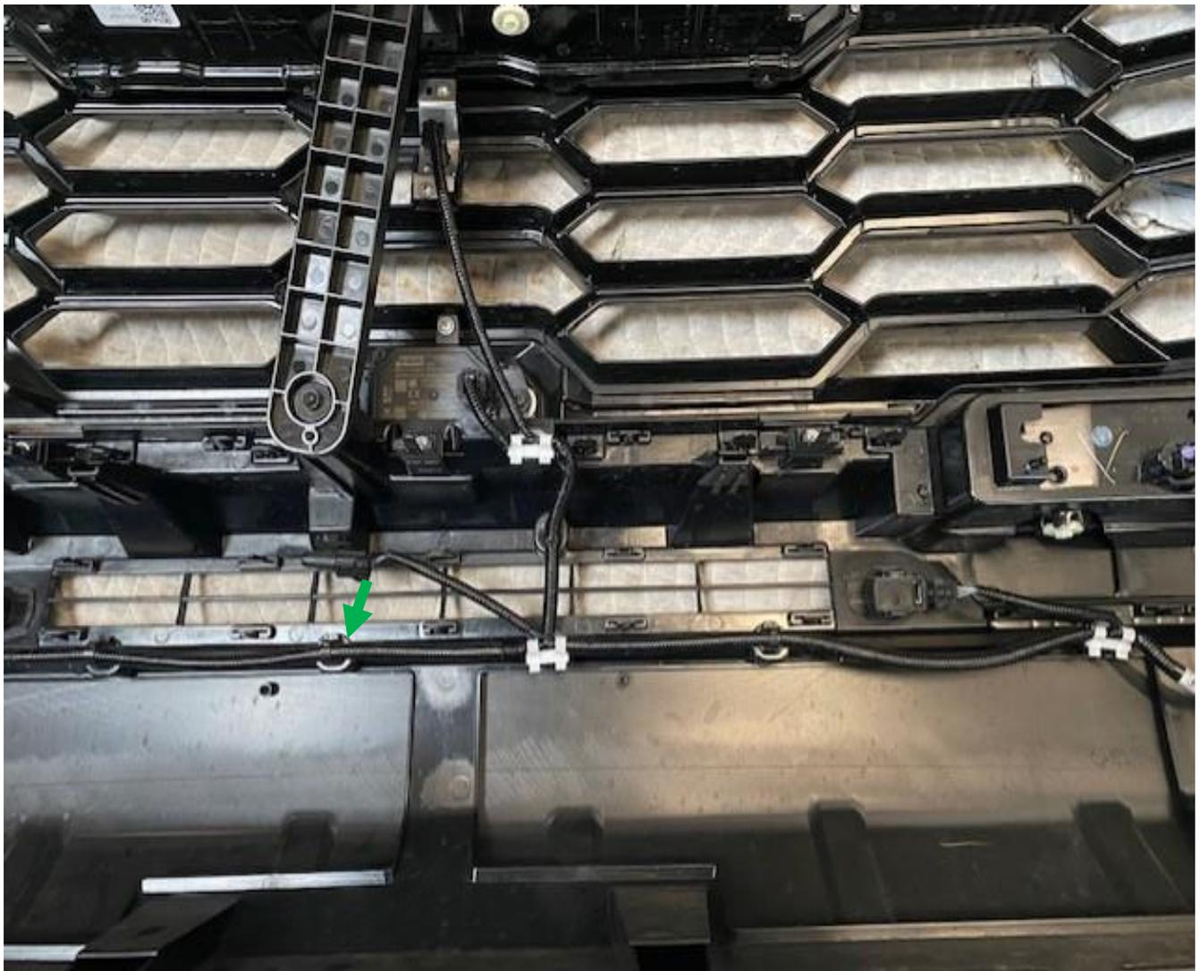
After: (TRD Pro Grill with Camera Wiring on Driver's Side)
