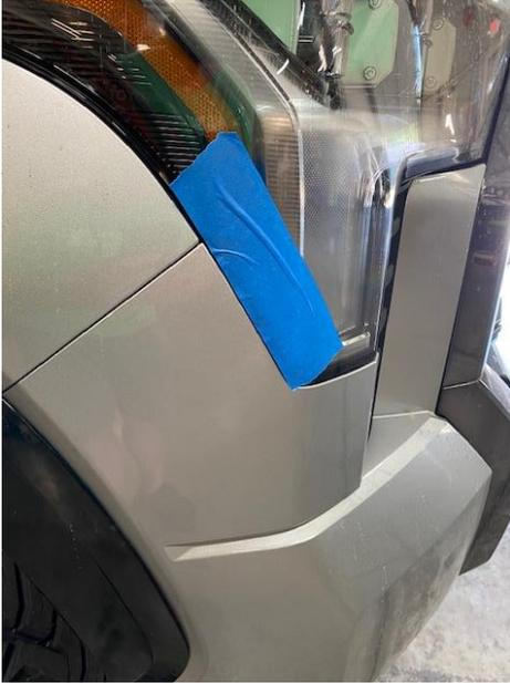
3. Remove 6 inner fender screws per side all the way up to the one above the centerline of the front wheel. Place the screws in a safe place or bag for reinstallation.
