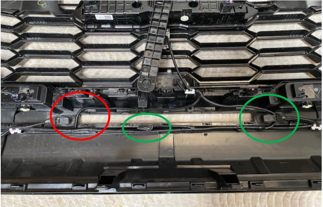
13. Loom and tape over the wires that have been re-routed to make the wires have a factory appearance and protection.
