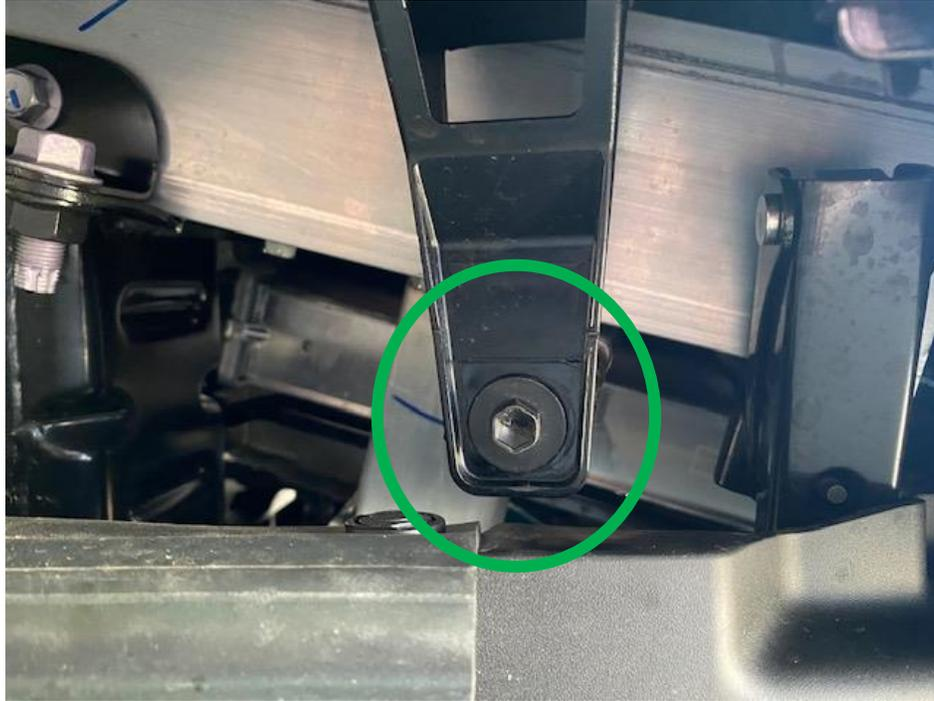
9. Remove the four bolts at the top of the front clip, these can be placed in the hole in the core support to make it easy to secure the front clip upon re-installation.
