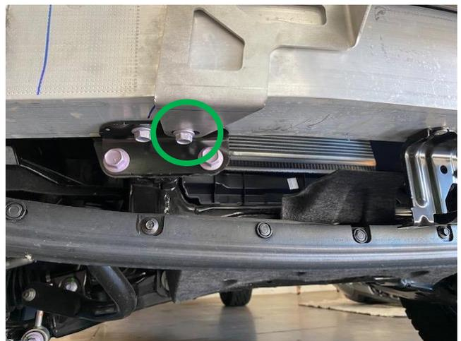
16. Install the light bar to the brackets loosely, each company will have a different mounting method, see the manufacturer's instructions. Make sure light bar wire is above the mounts before fully installing.
